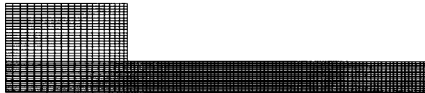
Fig. 10 Computational grid used for the sharp-edged orifice
