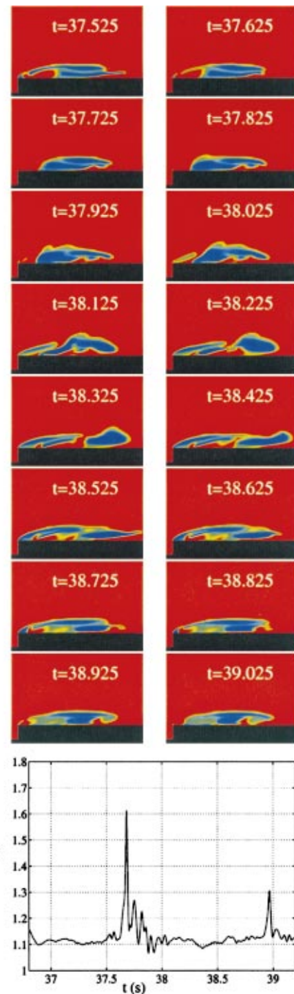
Fig. 6 Modeled flow over a 0-caliber ogive. Liquid volume fraction contours (red, \alpha_l > 0.995 ; blue, \alpha_l < 0.005 ) and corresponding drag history. UNCLE-M result. \sigma=0.3 . Re_D=1.46 \times 10^5 . D/U_\infty=0.146 (s), physical time step, \Delta t=0.001 (s).
